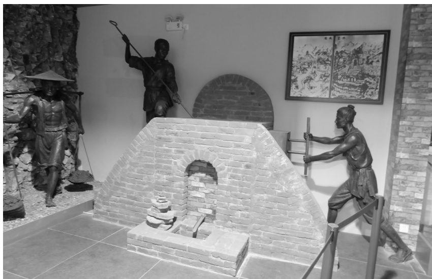
FIGURE 5. Model of a tin furnace in the early twentieth century in the Yunnan Tin Group Museum. Compared to textual sources, this model underrepresented the labor needed to operate the bellows. There should be two to three people instead of one operating the box bellows. Photo by Yijun Wang, 2016.
