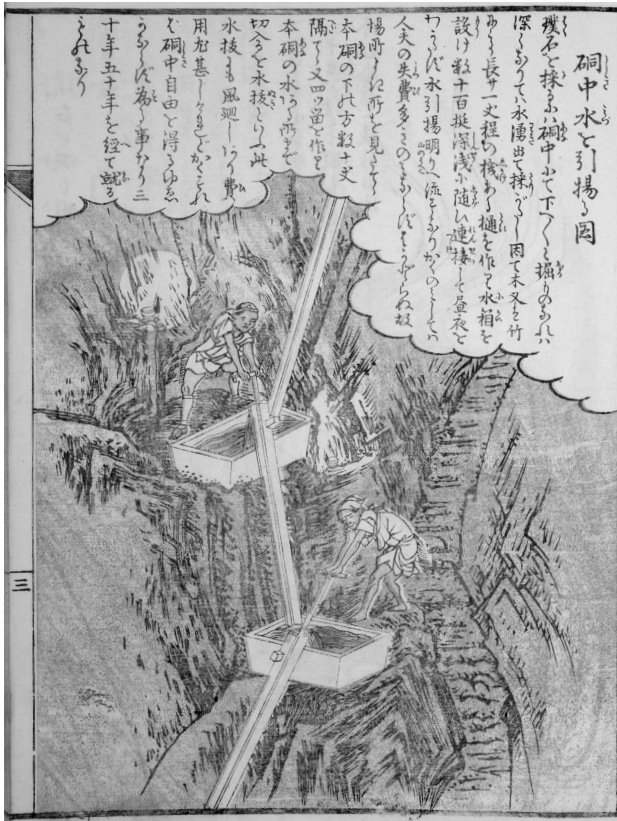
FIGURE 7. Water pumps in a Japanese copper mine, showing miners operating a vertical pump system of at least three interconnected levels. The structure of the pumps and the operation are extremely similar to those in Yunnan. Masuda Kō, Kodō zuroku (1795), 3a. Illustration by Niwa Tōkei. Woodblock print. 13.6 × 18.1 cm. Courtesy of the East Asian Library, Princeton University Library.
