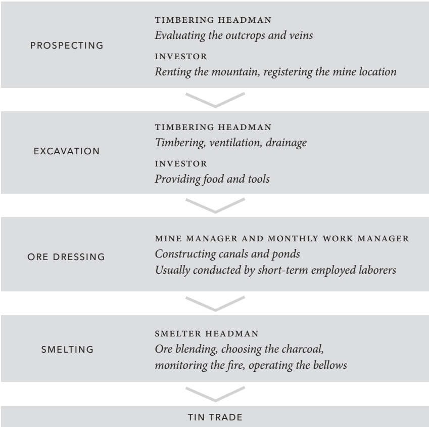
FIGURE 3. The production process of tin mining and smelting, showing the tasks and skills involved in each stage of production.
